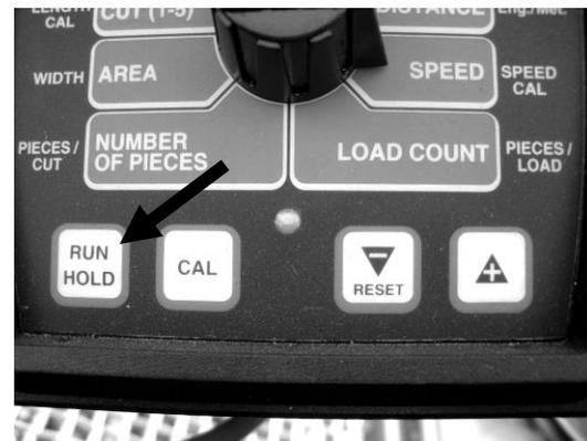
**Figure 2—RUN/HOLD button on Magnum II counter.**
