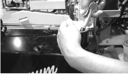
Figure 4—Apply light pressure to the fuel tank as shown.
