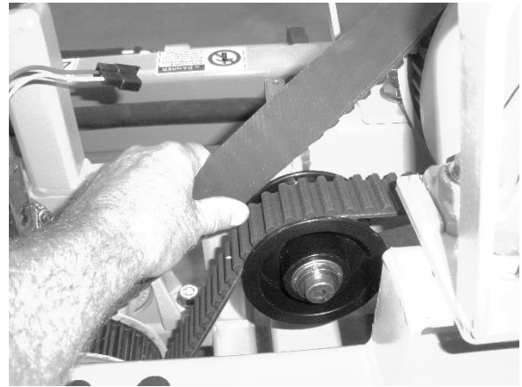
Figure 4—The belt has the correct tension when you can turn it one quarter turn using moderate force.
