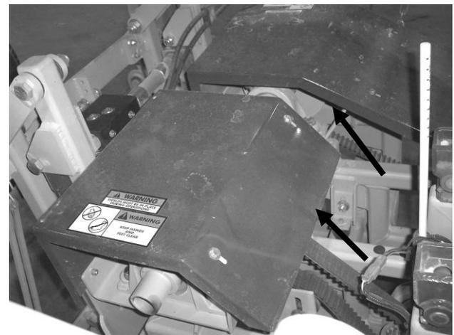
**Figure 2—Cutter Head Shields**
