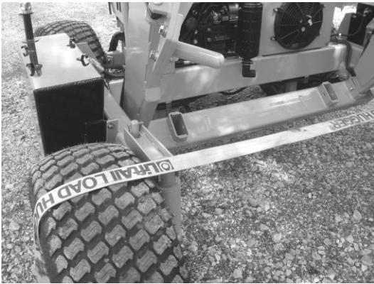
Figure 4—The front of the machine can be secured using a ratcheting strap placed over the tires.
