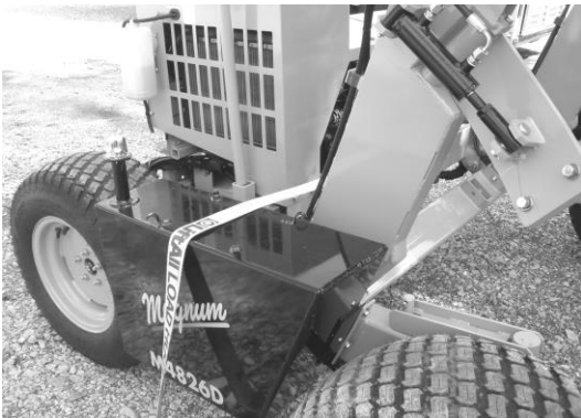
Figure 1—DO NOT strap the machine down using the fuel and hydraulic tanks.
