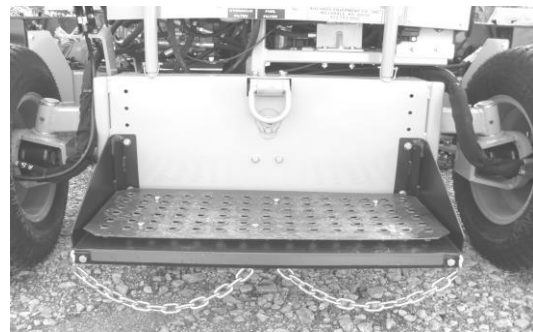
Figure 2—To prevent damage to the platform, do not use the chains to secure the machine on a trailer or truck.
