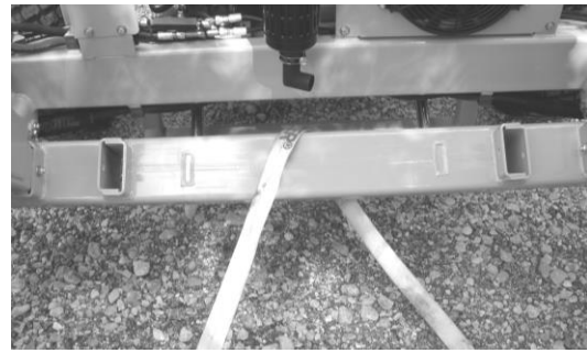
Figure 6—If necessary, place a strap around the roll lift frame and tighten it securely.
