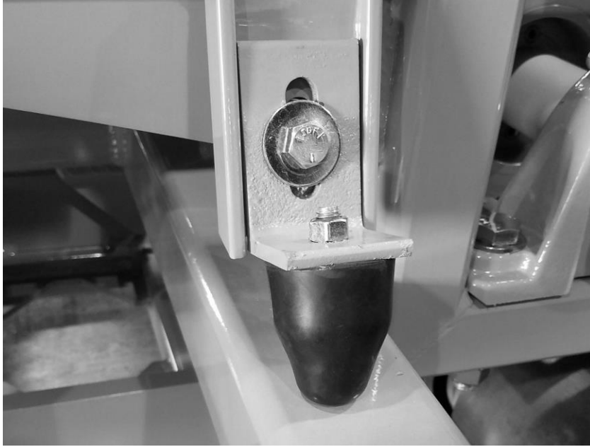
Figure 6 —The cutter head bumpers should be in firm contact with the harvester main frame.
