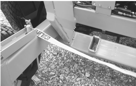
Figure 5—If necessary, raise the roll lift arms and secure the machine using a ratcheting strap across the main frame as shown.
