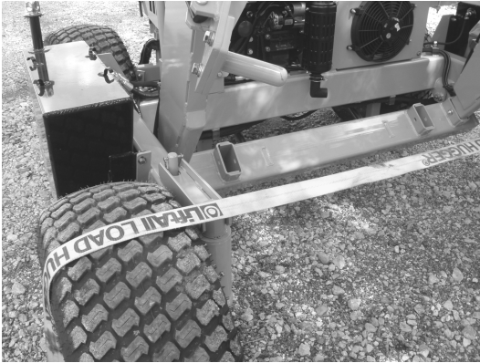
Figure 4—The front of the machine can be secured using a ratcheting strap placed over the tires.
