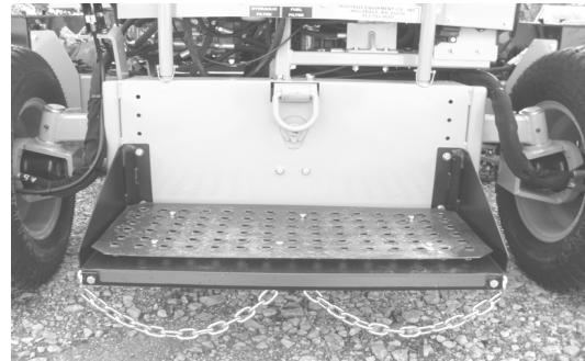
Figure 2—To prevent damage to the platform, do not use the chains to secure the machine on a trailer or truck.
