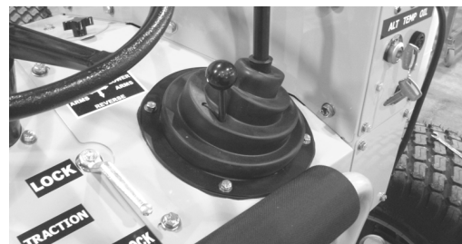
Figure 7—Remove the boot to access the control lever rod ends.
